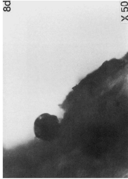
Figure 8 Optical microscopy photographs of unmodified and uncross-linked phenolic resin-coated sawdust-filled PP composite (composition 02 in Table I): (a) no external strain; (b) after 2% elongation; (c) after elongation to breaking point; (d) failure surface.
