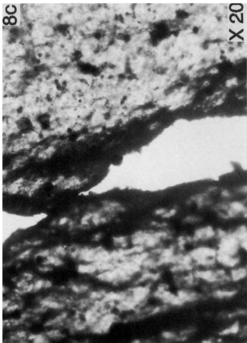
Figure 8 Optical microscopy photographs of unmodified and uncross-linked phenolic resin-coated sawdust-filled PP composite (composition 02 in Table I): (a) no external strain; (b) after 2% elongation; (c) after elongation to breaking point; (d) failure surface.
