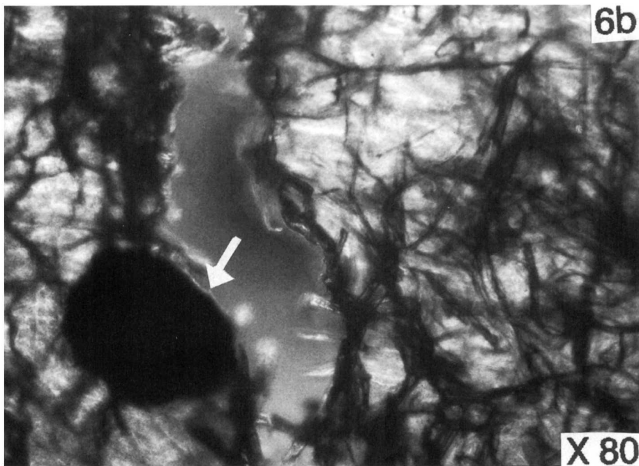
Figure 6 Optical microscopy photographs of unmodified V-pulp-filled PP composite (PP/V-pulp, 70/30): (a) no externally applied strain; (b) after an externally applied strain of 5% (very close to the breaking strain).
